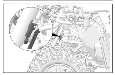
2. Route red and black wires up through opening in body panel marked "WINCH." Attach wires to body using push pin clip.
