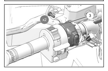
2. Connect handlebar switch ③ connector to vehicle main wire harness.
