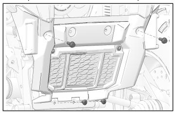
2. Remove two push pin rivets from panel on front bumper cover. Remove panel.
