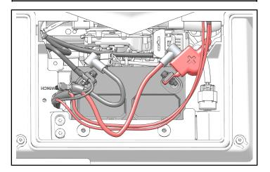
2. Make sure there are no exposed wires or terminals. Tightly bind all loose wires and attach away from moving parts and heat sources.
