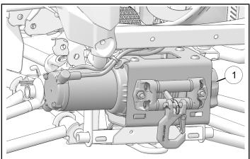
3. Attach winch to chassis using four screws ②. Torque to specification.
