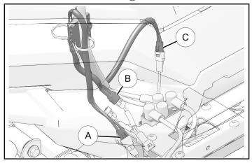
Route power wires for the Autostop control to battery area and connect orange wire to orange wire on the vehicle's main wire harness. Put black wires from control box to black (ground) terminal area.
