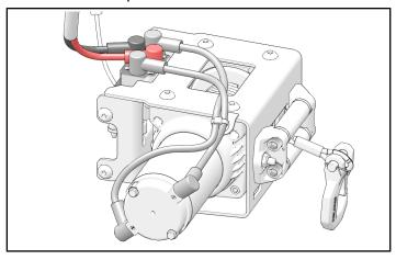
2. Put red and white wires through winch opening. put winch in position on chassis mount.
