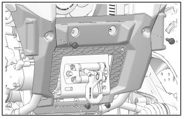
Close front rack and attach two rubber latches.
