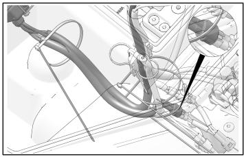
Route power wires for remote receiver to battery area and connect orange wire to orange wire on vehicle main harness. Route black wires from remote receiver to black terminal area.
