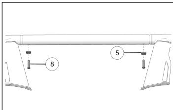
2. Align upper brush guard assembly ① on bumper.
