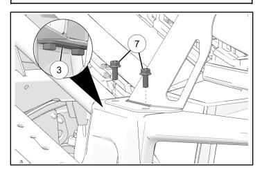
5. Torque four screws ① to specification.
