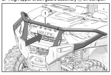
3. Loosely attach sides of brush guard with nut plate 9 and two screws 6.
